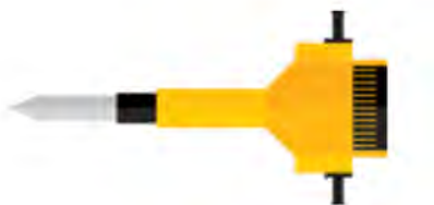
Impact driver with 3/8 Hex. Bit for type 14 gauges— Tek crew 5/16 Hex
